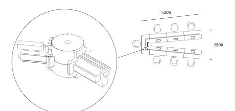
The free angle connector allows connection of two beams at multiple angles.
